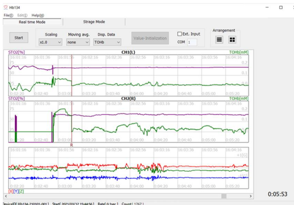
Figure 20. An example of corrected trend graph after inserting an initial value reset point (readout cursor).
