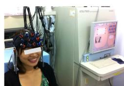
**Figure 2.** a whole-head type fNIRS measurement (Hitachi Med. ETG-7100)
