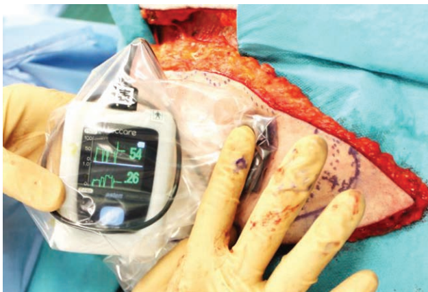
Fig. 1. A Toccare device showing the StO 2 value on its display. The module is light (0.1 kg) and runs on batteries. The sampling time is very short (0.5 s).
