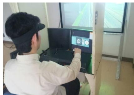
Fig. 3 Experimental set-up using train simulator. Participants join the driving experiment with wearable NIRS.
