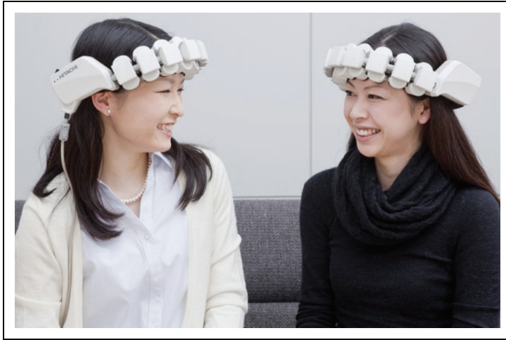
Figure 5. Mapping of the prefrontal cortex activity during face-to-face conversation by two wearable functional near-infrared spectroscopy (fNIRS) systems, each equipped with 22 channels (WOT-220, Hitachi High-Technologies Corporation, Japan). Each flexible probe unit covers the head in correspondence of the underlying dorsolateral and the rostral prefrontal cortex. The processing unit is worn on the waist. Multiple subject measurement (up to four people) is allowed. Photo courtesy of Hitachi.
