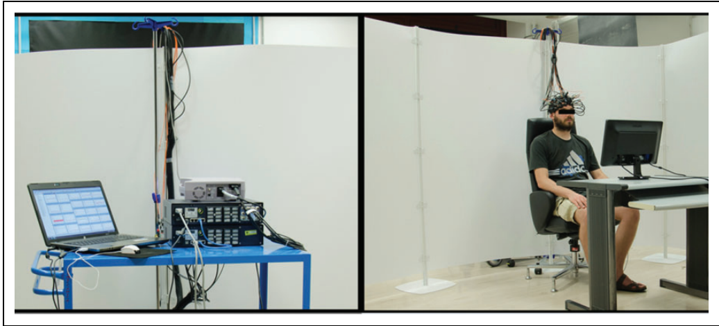
Figure 3. Example of a functional near-infrared spectroscopy (fNIRS) experimental setting. The subject is sitting in a comfortable high-backed chair. The illuminating optic fiber bundles and the collecting ones are assembled into a flexible probe holder fixed to the head by a Velcro brand fastener, adapting it to the size and shape of the head. The fNIRS instrumentation (Oxymon Mk III, Artinis, The Netherlands) is isolated from the subject by a white screen.
