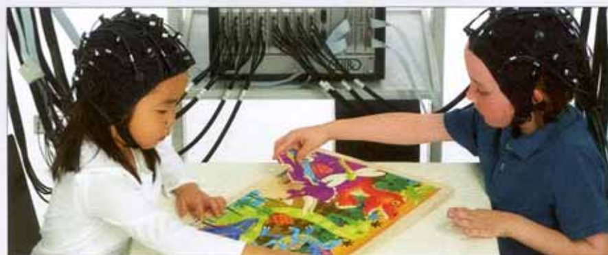
Figure 6. "Hyperscanning" measurement performed in two children playing with a puzzle (NIRScout extended, NIRx Medical Technologies, LLC, USA). Photo courtesy of NIRx Medical Technologies.
