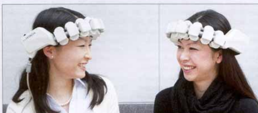
Figure 5. 22-channel wearable fNIRS system (WOT-220, Hitachi High-Technologies Corporation, Japan) mapping the prefrontal cortex activity. The flexible probe unit covers the dorsolateral and the rostral prefrontal cortex. The processing unit is worn on the waist. Multiple people measurement (up to four people) is possible. Photo courtesy of Hitachi.
