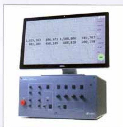
Figure 9. Commercial DCS NIR system: MetaOx (ISS, USA). The instrument provides concomitant measurements of O_2 Hb/HHb concentrations and Hb saturation (using frequency-domain NIR spectroscopy) and rCBF (using DCS) of the newborn head. The instrument can also monitor regional cerebral oxygen consumption. Photo courtesy of ISS.
