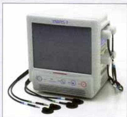
Figure 7. Time-domain brain NIR oximeter: tNIRS-1 (Hamamatsu Photonics Systems Division, Japan). The instrument is equipped with two optical probes. Photo courtesy of Hamamatsu.
