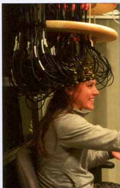
Figure 3. High density DOT optical fibre array covering two-thirds of the head. Photo courtesy of Professor Culver, Washington School of Medicine, St Louis, Missouri, USA.
