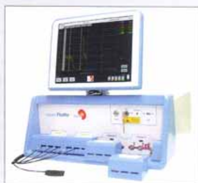
Figure 8. Commercial DCS NIR system for measuring the adult head rCBF: \alpha FloMo (Hamophotonics S.L., Spain). Photo courtesy of Hamophotonics.
