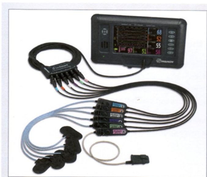
Figure 1. Commercial brain NIR oximeter: "SenSmart™ Universal Oximetry System" (Nonin). The NIR spectroscopy oximeter is equipped with five optical probes for monitoring the tissue Hb saturation over the forehead or in other parts of the body. Photo courtesy of Nonin Medical, Inc., USA.
