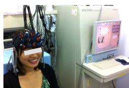
**Figure 2.** a whole-head type fNIRS measurement (Hitachi Med. ETG-7100)
